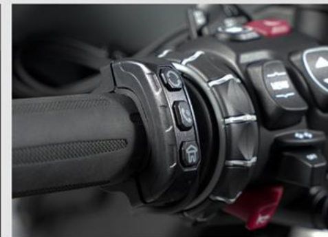
Handlebar Wire Controller Operation/车把线控器
